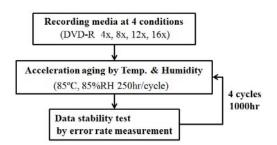
Figure 2. Experimental procedure for the stability test.
