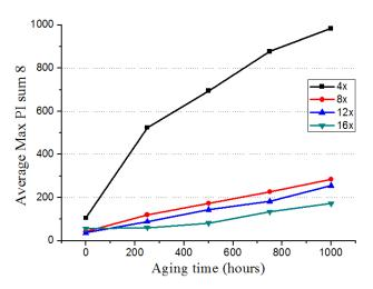
Figure 4. The average PI sum 8 value of DVD-R media as a function of recording speed after the acceleration aging test at the sever condition of 85°C/85%RH.
