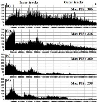
200000 400000 600000 1000000 1200000 1400000 1600000 1800000 2000000 2200000 Figure 5. The PI8 evaluation results for the media recorded at (a)4x, (b)8x, (c)12x, (d)16x after acceleration aging test.
