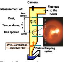
Figure 1. Experimental arrangement at the BRENDA combustion chamber.
