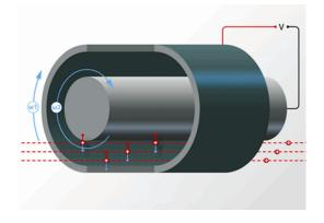
Figure 1: CPMA Principle:  $\omega_2 > \omega_1$
