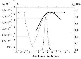
Fig. 2 The axial profiles of supersaturation ratio (S), homogeneous nucleation rate  $(J_{cl})$  and schematic function of the outlet number concentration of aerosol during "cut-off" experiments. The "0" position corresponds to the geometric end of the heater.
