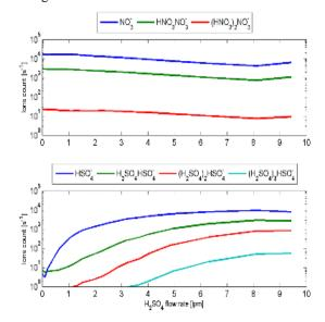
Figure 1. Sulfuric acid and reagent ion concentrations in CI-TOF-MS spectrum.
