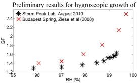
Figure 1. A comparison of growth factors (GF) for HULIS from SPL and Budapest, spring (Ziese et al, 2008).
