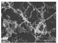
Figure 2. SEM image of soot produced by burning diesel fuel mixed with ferrocene.
