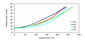
Figure 1. Pressure drop increase vs. loading time for samples A,B,C and D
