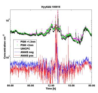
Figure 1. Example of measurements with PSM at cut-off sizes 1.3 and 2nm, compared to TSI 3786 (UWCPC) at 3nm cut-off and small positive and negative ions measured with ANAIS ion spectrometer.
