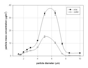
Figure 3. Particle mass concentration of axial-flow cyclone inlet and outlet.
