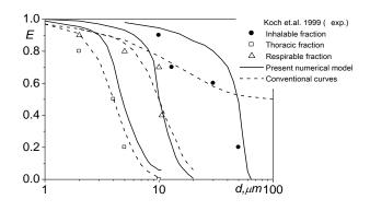
Figure 2. Collection efficiencies of RespiCon stages as a particle diameter function
