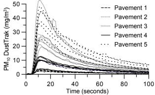
Figure 1. PM10 concentration in the measuring chamber during the test cycle.
