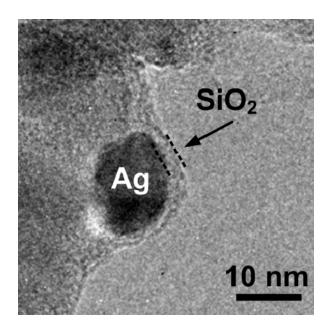
Figure 1. TEM image of the composite  $Ag/Fe_2O_3 SiO_2$ coated nanoparticles. The silver nanoparticle (dark particle) is attached on the iron oxide core, and encapsulated by a nanothin silica layer of about 2 nm thickness.
