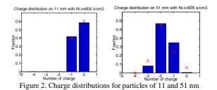
The zone of mixing is axi-symmetric. Radial and axial profiles of ion density are stationary but asymmetrical. Simple estimations of these profiles have been done, but angular profile depends on gas velocity and possible surface or space charge effects. Measured charge distributions are broader than calculated ones proving that particles encounter different charging conditions.
