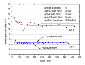
Figure 1. Long term stability and reproducibility of mean particles sizes (SMPS-measurement)
