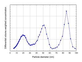
Figure 1. Simultaneous measurement of 20, 50, and 83 nm PSL spheres using the ultrafine nebuliser (Van Schooneveld *et al.*, 2010).
