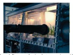
Figure 1. Exposure of maize plants to a cerium oxide aerosol in an enclosed cabinet (glove-box).
