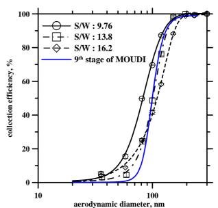
Figure 2 Calibration results of the present micro-orifice impactor.
