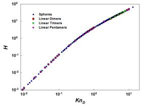
**Figure 1.**  $H(Kn_D)$  relation from mean hitting time calculations. Particles of all shape collapse to a single curve.
