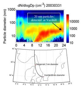
Figure 1. The observed particle number size distribution March 31, 2003 during a formation event at the Vavihill site (upper panel). The detected 20 nm diameter particles at Vavihill around 23:00 hours can be traced back to the time when they were formed as 2 nm particles 13 hours earlier over the Skagerrak sea (lower panel showing the
