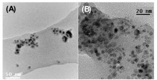
Figure 2. TEM images of  $Si/SiO_2$  coated copper core particles formed at 800 (A) in nitrogen and (B)  $H_2/N_2$  atmosphere.
