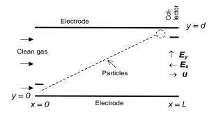
Figure 1. Schematic representation of the DMA.
