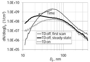
Figure 1. The non-volatile (TD (thermodenuder) on) and semi-volatile (TD off) particle size distributions during the medium load point with the S350 fuel.
