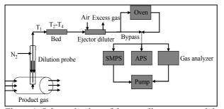
Figure 1. Schematic view of the sampling system and the battery of aerosol instruments.
