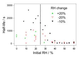
Figure 1. Timescales, represented as half-lives, for equilibration of sucrose particles, for both increasing and decreasing RH steps. The glass transition ( $\sim 25\%$  RH) is represented by the dashed line.
