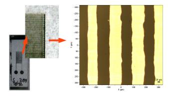
Figure 2: Interdigital electrodes made of silver on a glass substrate.
