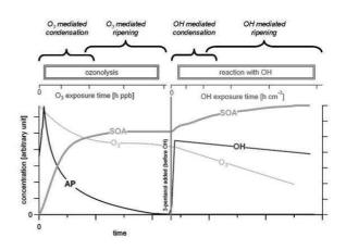
Figure 1. Four phases of transformations of secondary organic aerosol (SOA) from α-pinene (AP) as observed during ozonolysis and OH exposure.
