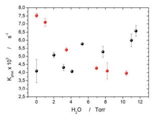
Fig. 1. Dependence of photolysis rate on water vapour concentration: black dots – benzaldehyde, red dots – salicylic aldehyde.
