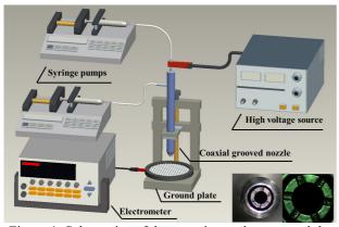
Figure 1. Schematics of the experimental set-up and the nozzle geometry.
