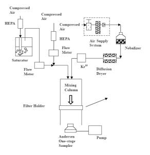
Figure 1. The experimental test setups.
