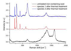
Figure 1. Raman spectrum of iron-containing soot untreated and thermally treated.
