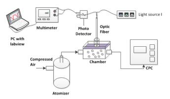
Figure 1. Schematic of experiment set-up
