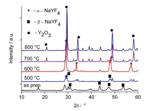
Figure 2. XRD patterns of the NaYF<sub>4</sub>: Yb, Tm powders sintered at different temperatures.
