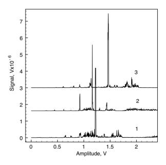
Figure 2. QCM measurements with different rates of gas flow through the generator for constant W fila - ment temperature, curve 1 - chosen conditions, curve 2 - air flow decreased by 10%, and curve 3 - air flow in-creased by 10%.
