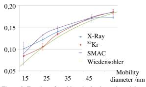
Figure 2. Fraction of positive single charged particles produced by the different chargers
