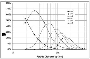
Figure : Charging efficiency as function of particle size for charge fraction from 0 to 5
