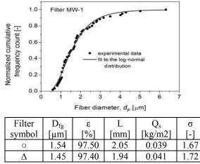
Fig. 1. Fiber size distribution and filter characteristics
