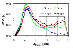
Figure 1 q<sub>3</sub> Aerodynamic particle size distribution of AC fine (ISO 12103-1) for different nozzle sizes
