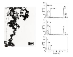
Figure 1. *Left* – TEM image of a particle aggregate formed in the tertiary vapour experiments described. *Right* – EDX spectra of olivine particles of varying Fe-Mg composition
