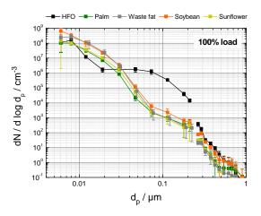
Figure 1. Number size distribution of particles emitted from a marine Diesel engine operating on different biofuels and on heavy fuel oil (HFO) as a reference case.
