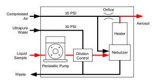
Figure 2. Flow schematic of the ultrafine nebuliser.
