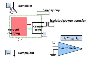
Figure 1. Schematic of sensor operating principle.
