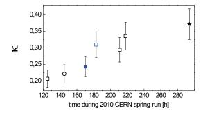
Figure 1. The figure illustrates derived κ-values from CCN activation measurements for different initial experimental conditions of different runs during the CLOUD Spring campaign 2010. Open symbols represent charged pion beam conditions, filled symbols neutral conditions, black symbols low relative humidity and blue symbols higher relative humidity conditions at CLOUD chamber temperature of 20°C. Star symbol represents
