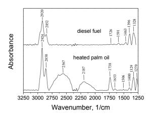
Figure 1. IR spectra of particles produced by burning diesel fuel and heated palm oil by a Zetor tractor engine.
