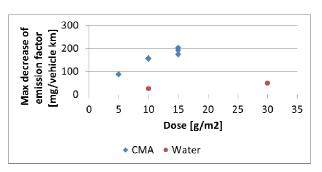
Figure 3. The absolute maximum decrease of the emission factor assuming a constant deposition velocity in the room. A normal emission factor for the studded tyre setup is between 290 and 570 mg/vehicle km.
