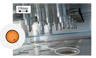
Fig 1: ten nozzles spraying head / Deposit on the patch
