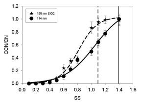
Figure 1. Activation curves from CCN counter. The data are not corrected for shape or multiple charges in the DMA.
