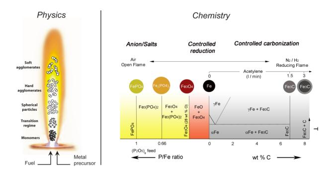
Figure 1: Physical understanding of particle formation in a gas stream (left) and the variety of chemical compositions (right) of nanoparticles (present example: iron) prepared by flame spray synthesis are shown.
