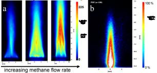
Figure 2. a) OH chemiluminescence images of the flame with increasing methane flow rate (from left to right); b) probability density function of 100 Mie scattering images
