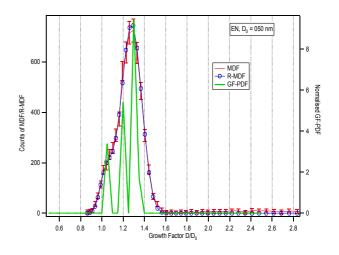
Figure 2. GF-PDF fitting result of 50nm ambient aerosols
