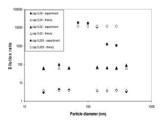
Figure 1. A comparison between dilution ratios determined experimentally and predicted theoretically.
