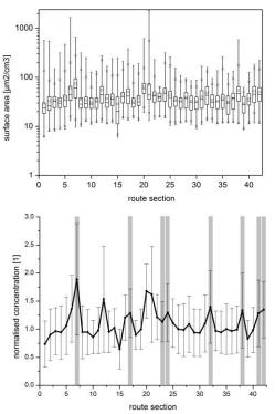
Fig 1 Top: Alveolar lung deposited surface area concentrations along 42 route section in Braunschweig, Germany. The plot indicates the mean (circles), median, 25 and 75 percentile (box), 1 and 99 percentile (asterisks) and absolute minimum and maximum (whiskers). Bottom: Mean normalised ALDSA during 15 measurements at the route sections. The high density traffic sections are indicated by grey shadings.
