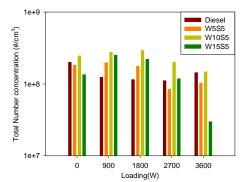
Figure 1.Total number concentration of exhaust from a diesel engine generator as different fuel and loading.
