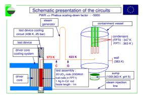
Figure 1. Schematic of Phebus experiments FPT0 and FPT1 showing aerosol source, circuit and model containment vessel with internals
