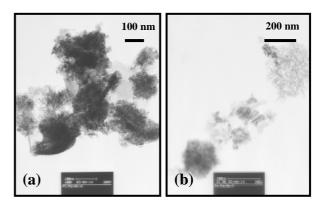
Figure 2. TEM photograph of (a) fresh and (b) after activity test Pt-Pd-Rh nanoparticles cordierite substrate catalyst. Test conditions: 800 ppm NH<sub>3</sub> in He,  $O_2=4\%$ , GHSV=92000 hr<sup>-1</sup>.
