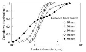
Figure 1. Cumulative size distribution of dry ice particles exhausted from nozzle (nozzle diameter = 0.2 mm).
