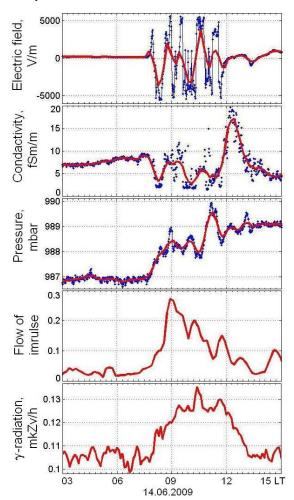
Figure. Coordinated variations of atmospheric electrical, meteorological values and gamma-background in storm atmosphere.
