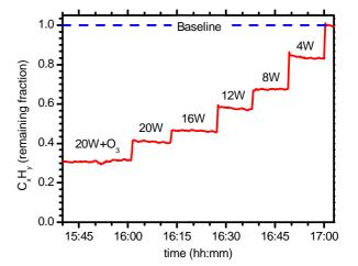
Figure 1. Reduction of HC for different UV light intensities (85% at 254nm and 15% at 185nm) and for UV plus O<sub>3</sub> from a corona wire. Residence time 1s.
