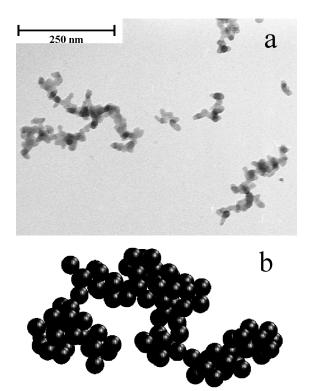
Figure 1: (a) Soot sampled from a flame. (b) Modelled soot particle.
