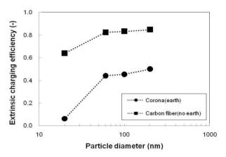
Figure 1. Comparison of extrinsic charging efficiency with particle diameter for carbon fiber and stainless steel corona chargers.
