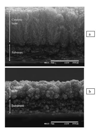
Figure. Cross-sectional SEM micrographs of the profiles of electrosprayed Pt/C catalytic layers over a carbon paper substrate (for the same catalyst loading). (a) fractal-like structures for a flow rate of 0.2 ml h<sup>-1</sup>, and (b) Deposits based on spheroids for 0.5 ml h<sup>-1</sup>. In both images the micron bar corresponds to 300  $\mu$ m.
