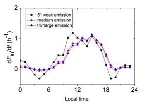
Fig. 2 Aging rate of soot particles due to condensation process
