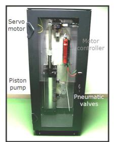
Figure 1. The pulmonary waveform generator
