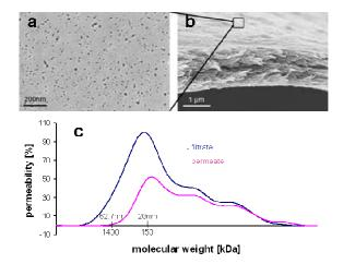
Figure 1: Top view on PES membrane with a MWCO of 150kDa (a). Cross section of the same membrane (b). Typical dextran rejection profile of a 1400kDa MWCO membrane (c).
