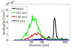
Figure 1. Size distributions of the TiO<sub>2</sub> agglomerates before impaction (intact) and the bounced particles
