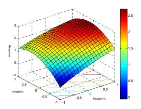
Figure 1: 3D plots of reaction yield of acids as a function of BSTFA and pyridine concentrations.
