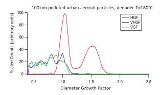
Figure 1. Hygroscopic Growth Factors (HGF), Volatility Growth Factors (VGF) and Hygroscopic Growth Factors of particles after passing through the thermal denuder (VHGF) of polluted urban aerosol at RH of 90%.
