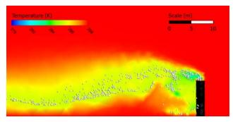
Figure 1. Model output for a single sea-going spraying device at a windspeed of 3 m/s from the right and neutral atmospheric stability. Gas phase temperatures are color coded and the dots represent ensembles of particles
