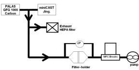
Figure 1. Experimental device of clogging of media by nanoparticles aggregates
