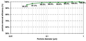
Figure 2. Bag filter submicron particles removal efficiency.
