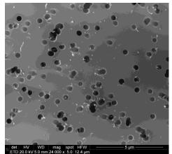
Figure 2. The SEM image of collected airborne MWCNTs with 75 nm mobility size.
