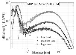
**Figure 1.** Non-volatile particle distributions measured with low, medium and high load. FIP=140 MPa, speed 1500 RPM
