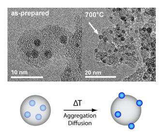
Figure 1. Morphological transformation of noble metal encapsulated in oxide nanoparticles to supported on oxide particles (2 vol% Pd with SiO<sub>2</sub> matrix).
