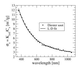
Fig.1: experimental spectrum of the specific extinction coefficient  $\sigma_s = \text{kext/Cs}$  of diester soot ( $\sigma_s = \text{kext/Cs}$ , with Cs the mass concentration). The continuous line represent the calculated values with the dispersion model of Lorentz-Drude
