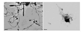
Figure 1. Electron Micrographs of a) 'long', bar =  $2 \mu m$ and b) 'tangled' CNT particles, bar =  $1 \mu m$ . Images kindly provided by Dr Craig Poland, IOM.
