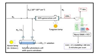
Figure 1. Schematic of experimental set-up used to study the reduction of  $IO_3^-$  to  $I^-$  and subsequent emission of  $I_{2.}^-$
