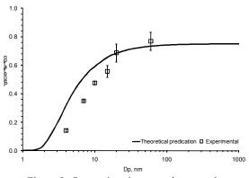
Figure 2. Comparison between theory and experimentally measured solid particle penetration.
