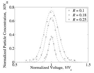
Figure 2: 296 nm PSL classified with a high resolution prototype CPMA; *R* is the resolution parameter.
