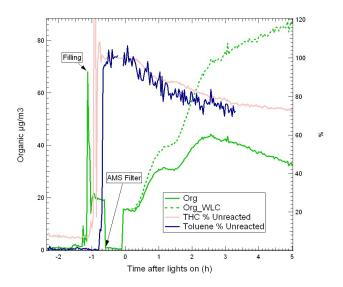
Figure 1: Time series from a smog chamber experiment on moped exhaust showing the evolution of organic aerosol concentrations together with the percentage of unreacted total hydrocarbons and toluene. The second observed increase in OA is due to the addition of NO to the smog chamber.
