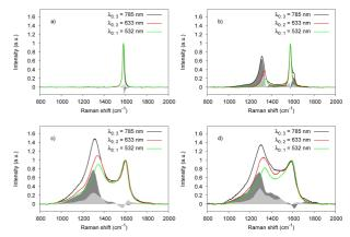
Figure 1. Raman spectra (at different  $\lambda_0$ ) of highly oriented pyrolytic graphite (a), graphite powder (b), diesel soot (c) and spark discharge soot (d) with corresponding difference spectra.
