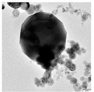
Figure 1 Freshly nucleated AISI 308 stainless steel aerosol. Primary particle size of magnetite and Ni-rich dendrites.
