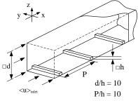
Figure 1. Experimental setup of periodic steps
