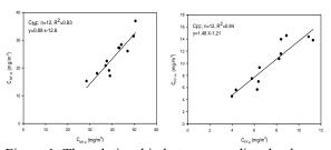
Figure 1. The relationship between predicted value  $(C_{NF-p} v.s C_{FF-p})$  and measured value  $(C_{NF-m} v.s C_{FF-m})$  were obtained by using Two-Zone model in the near and far field.
