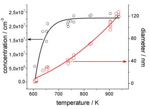
Figure 2. Aerosol concentration and aggregate size vs heating temperature.
