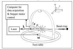
Figure 1: Schematic lay out of the scattering setup
