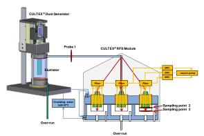
Figure 1: Schematic setup of the Cultex<sup>®</sup> RFS with three sampling points
