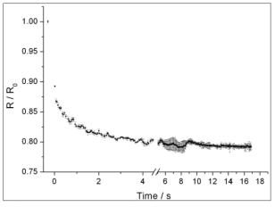
Figure 2. Water evaporation of 50:50 water / glycerol aerosol droplets in a dry gas flow (error bars indicate standard deviation of multiple droplets)
