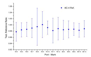
Figure 2. Radial uniformity of 55 nm soot particle concentration. The points span the central 30 cm of the chamber.
