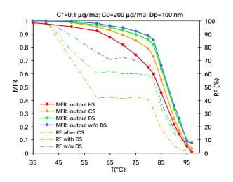
Figure 1. Mass fraction remaining (MFR) and recondensation fraction (RF) calculated for a standard thermodenuder system. HS=heating section (0.5 m), CS=cooling section (0.15 m), DS=denuder section (0.5 m). Tube diameter=0.022 m. Sample flow=0.6 lpm.
