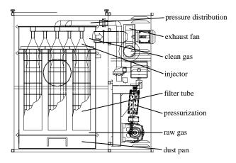
Figure 1. Prototype of the baghouse filter.
