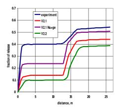
Figure 2. Exerimental and calculated deposition profiles of Molybenum along the circuit in FPT1
