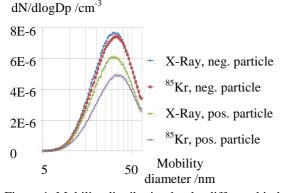
Figure 1. Mobility distribution by the different kind of chargers measured by a SMPS System
