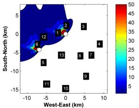
Fig. 1: Contours of ground level SPM - February 2010, 14:30 IST ( $\mu$ g m<sup>-3</sup>). The text markers denote measurement sites and large white markers the power stations.
