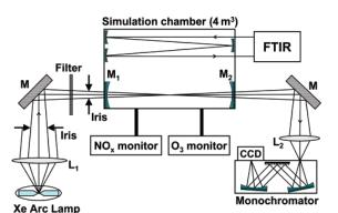
Figure 1. Schematic depiction of the coupling of the atmosphere simulation chamber and the IBBCEAS spectrometer (after Venables *et al.*, 2006).
