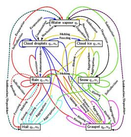
Figure 1. Simplified schematic diagram of the microphysical interactions in the two-moment Seifert scheme with respect to the particle classes cloud- and rain droplets, cloud ice, snow, graupel and hail.
