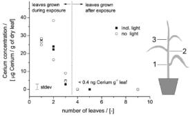
Figure 2. Cerium concentrations in plant leaves 3 months post nanoparticle exposure. Leaves 1-3 were directly exposed during the exposure, leaves 4-9 grew following the exposure.
