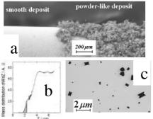
Fig. 1. Zn nucleation data a) SEM image of wall deposit, b) wall deposit axial profile, c) TEM images of the outlet particles. Nucleation temperature T =660 K.
