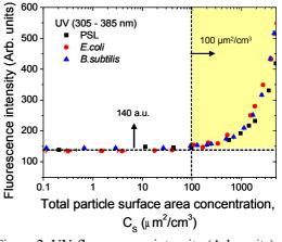
Figure 2. UV-fluorescence intensity (Arb. units) vs. particle concentration.
