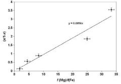
Figure 2. Correlation plot of the ratio of x/1-x (equivalent to measured Mg/Fe in particles) to the ratio of precursor flows used for particle generation.
