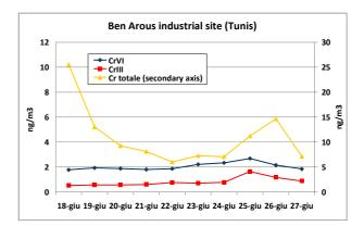
Figure 1. Total Cr (XRF determination), Cr(III) and Cr(VI) during a short monitoring campaign at the industrial site of Tunis
