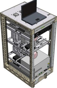
Figure 1. 3D-drawing of the Zeppelin-AMS-Rack.
