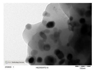
Figure 1: TEM-image of a electrostatic-precipitated polyurethan swarf particle with firmly embedded ZnO NPAs
