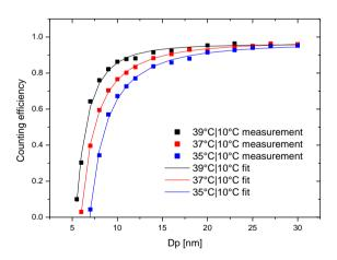
Figure 1: Counting efficiency of the Fast CPC (FCPC) at three temperature differences. Squares present mean values of three runs, the solid lines are fitted using the four-parameter equation:  $\eta = a - b/(exp(c*log(x))-d)$ .
