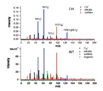
Figure 1. Average negative single particle mass spectra of cloud residual particles (top) and background aerosol particles (bottom) measured by ALABAMA
