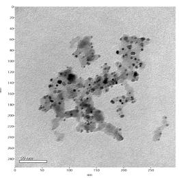
Figure 2. TEM images of Pt/Al<sub>2</sub>O<sub>3</sub> particles by MOCVS/MOCVD process
