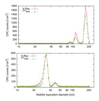
Figure 2: Efficiency of the soft X-ray charger compared with a radioactive <sup>241</sup>Am charger using monodisperse DEHS particles.
