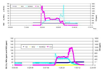
Figure 1. Gas composition during shutdown (up) and start-up transients (from and to 250MW)
