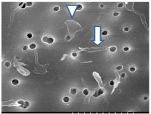
Figure 1 Bundle of SWCNT in the chamber
