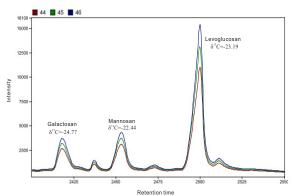
Figure 1. TD-2DGC-IRMS analysis of levoglucosan, mannosan and galactosan in softwood burning aerosol. Signals of  $\text{CO}_2^+$  (m/z 44, red), and isotopologues on m/z 45 (green), and m/z 46 (blue) are shown.
