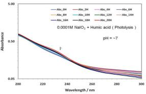
Figure 2.UV-visible spectra of a photolysed  $10^{-4}$ M NaIO<sub>3</sub> solution (+ Humic acid).
