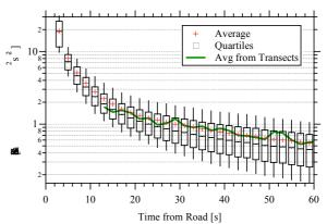
Figure 1. Turbulent kinetic energy measured at the roadside as a function of time from the road along the wind direction.
