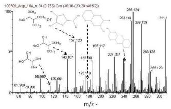
Figure 1. Examples of mass spectrum evidencing some products of glyoxal in aerosols from Aspyreten, Sweden.
