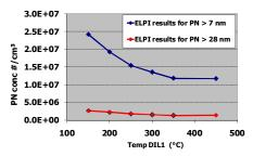
**Figure 1.** Number of particles from a marine diesel engine, measured by ELPI during increasing sample temperature.
