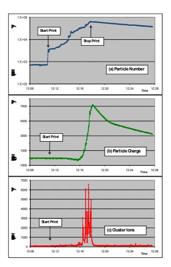
Figure 1: Time series of (a) PNC (b) CPC and (c) CIC in the chamber during a typical print run of 150 sheets.
