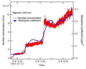
Figure 2. Real-time measurement of absorption coefficients and number concentrations.
