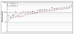
**Figure 1.** Recovery rate (%) of elements by burning wood-chips in a 30 kW boiler (combined element amounts in grate ash, internal heat exchanger ash, ESP ash and fly ash divided by the element amounts contained in the wood chips)
