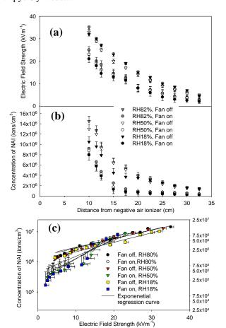
Fig. 1 The distance-dependent (a) electric field strength and (b) NAI concentration; (c) the liner relationship between the logarithm of NAI concentration and electric field strength
