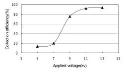
Figure2. Effect of applied voltage on collection efficiency.
