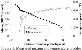
figure 1. Measured mixing and temperature profiles in the diluting probe.
