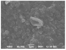
Fig. 2: Scanning Electron Microscopy (SEM) of a leaf sample from a monitoring station at NLC showing particle aggregates from power plant emissions.
