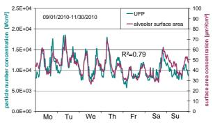
Fig. 1: Particle surface area (NSAM) and UFP (SMPS) concentration of the ambient aerosol for summer and autumn 2010.
