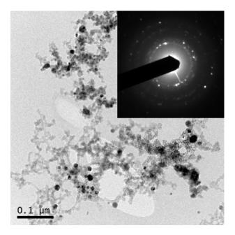
Figure 1. HRTEM image and SAED pattern of particles prepared at  $T_{\rm R}$ =700°C,  $c_{\rm O}$ =10 vol. %,  $P_{\rm COAA}$ =0.32 Pa,  $P_{\rm TEOS}$ =1.89 Pa,  $Q_{\rm R}$ =800 cm<sup>3</sup>/min.
