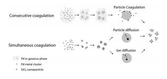
Figure 2. Possible 2-component nanocomposite formation mechanisms in flame spray synthesis.
