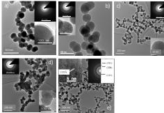
Figure 1. HR-TEM micrographs and SAED diffraction patterns of the produced particles at different temperatures: a) T = 800 °C, b) T = 900 °C, c) T = 1000 °C, d) T = 1200 °C and e) 1400 °C
