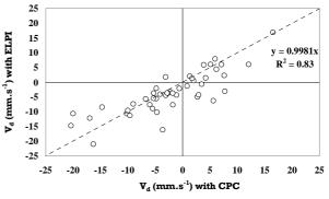
Figure 1. Dry deposition velocity measured with an ELPI and a CPC.
