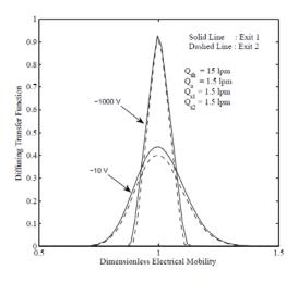
**Figure 1**. Transfer Function of the DMO-DMA for which the first sample exit is located at distance 44.369 cm downstream the inlet, while the second at distance 4.987 cm. The outer radius of the apparatus is 1.961 cm and the inner radius is 0.937 cm.
