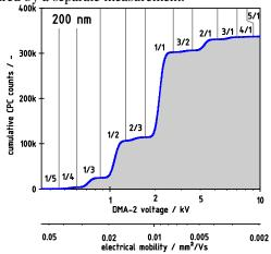
Figure 2. cumulative particle counts of the aerosol introduced in Fig. 1 when performing an up-scan using a logarithmic voltage ramp
