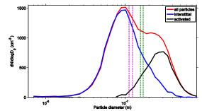
Figure 1. Size distributions of all particles (red), interstitial particles (blue), and activated particles (black). Green and purple dotted lines represent the range of the critical diameter ( $D_{50}$ ) derived from the CCNc data during the cloud event, for SS=0.1% and SS=0.2% respectively.
