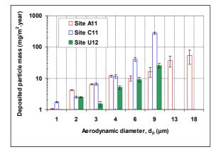
Figure 1: Comparison of deposited particle mass flux at horizontal surfaces in ventilation air supply ducts for the three industrial sites.
