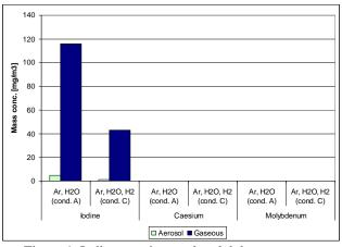
Figure 1. Iodine, caesium and molybdenum mass concentrations in the second experiment, calculated from aerosol filters and bubbling bottle ICP-MS data.
