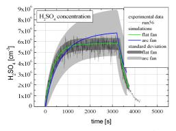
Figure 1: Simulated temporal evolution of the  $H_2SO_4$ concentration in the CLOUD chamber compared to  $H_2SO_4$  lifetime experiments. Simulations shown here were carried out for different fan shapes, but for equal  $H_2SO_4$  production rates (4e5 cm<sup>-3</sup>s<sup>-1</sup>).
