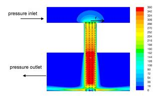
Figure 1. Velocity contours in the LPI nozzle. Particles and their tracks are schematically marked in the figure.
