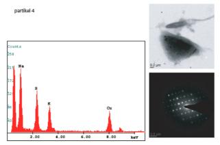
Figure 1. EDS spectrum (left) and TEM bright field image (top right) with selected area electron diffraction pattern (bottom right) of a sodium rich aphtitalite particle (triangle) sampled on top of Stromboli volcano.
