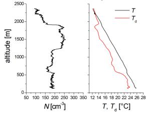
Figure 1. Vertical profiles of total particle number concentration (N), temperature (T) and dewpoint ( $T_d$ ) during RF9.
