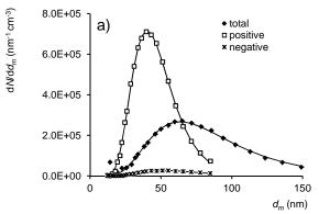
Figure 1. Positively and negatively self-charged Mg particles in purified gas and the total size distribution measured with a neutralizer, at a capacitor charging current of 9 mA. Lines represent lognormal fits to the data.
