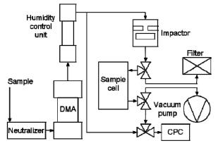
Figure 1 Schematic representation of measurement system
