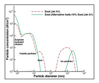
Figure 2. Simulated size distributions of particles in the aircraft plume at ~125 m behind the plane with standard fuel (red dashed) and alternative fuel (green solid).
