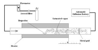
Fig. 1 The scheme of the flow chamber.
