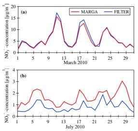
**Figure 1**. Nitrate measurements in  $PM_{10}$ . Comparison of daily High-Volume filter measurements (quartz-fibre filter, DIGITEL DHA-80, blue line) with MARGA measurements (red line) in (a) March 2010 and (b) July 2010.
