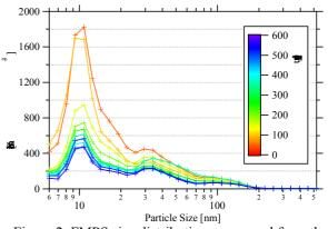
Figure 2. FMPS size distributions measured from the mobile lab binned by time from the road along the wind direction.
