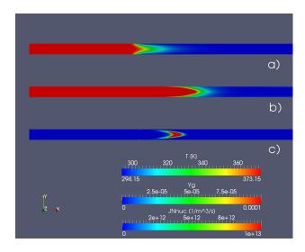
Figure 1: Snapshots from a laminar simulation of dibutyl phthalate: temperature field T[K] (a), species mass concentration in the gas phase  $Y_g[kg/kg]$  (b) and nucleation rate  $J_N[m^{-3}s^{-1}]$  (c).
