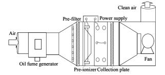
Figure1. Schematic diagram of the pilot scale ESP system
