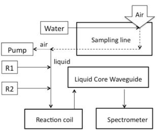
Figure 1. Scheme of the instrument. R1 and R2 denote the reagents phenol and hypochlorite.
