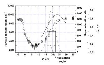
**Fig. 3.** Outlet concentration of aerosol particles (circles) as a function of the grid coordinate *Z*, the axial profiles of supersaturation (solid line) and reference nucleation rate  $J_{cl}$ , evaluated via the classical formula (dashed line).
