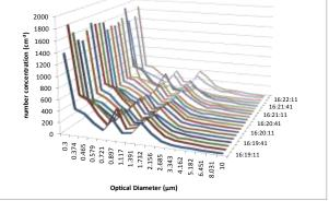
Figure 1: Atmospheric aerosol measured with the OPS 3330 in January 2011.
