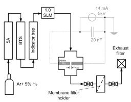
Figure 1. Spark discharge setup.
