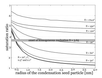
Figure 1: Heterogeneous onset curves for water at T = 285 K. Each point on the curves corresponds to a nucleation probability of P = 1/2 with an indicated contact angle in the (R,S)-plane. The onset of homogeneous nucleation, S = 3.65, is marked with a grey bar.
