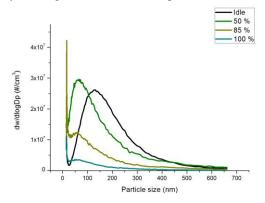
Figure 1. Size distribution of particles emitted in the interval 15-680 nm as a function of engine load.
