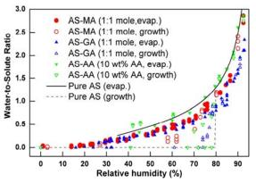
Figure 2. Hygroscopic properties (water-to-solute mass ratio) of pure AS and AS-organic mixed particles.
