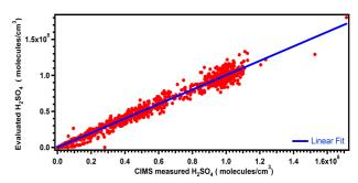
Figure 1. Example of the correlation between the evaluated  $[H_2SO_4]$  from the growth rate and the  $[H_2SO_4]$  measured by CIMS.
