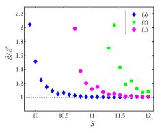
Figure 1: Ratio of apparent and true critical sizes for water at 260 K with three monodisperse background aerosol distributions: (a) diameter  $d_p = 100$  nm and number concentration N = 10000 m<sup>-3</sup>, (b)  $d_p = 10 \ \mu$ m and N = 10000 m<sup>-3</sup>, and (c)  $d_p = 10 \ \mu$ m and N = 1000 m<sup>-3</sup>.
