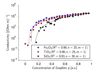
Figure 1: Electrical conductivity of graphite with admixtures of  $SiO_2$ ,  $TiO_2$  and  $Fe_2O_3$  nanoparticles. The data is fitted by the percolation theory.
