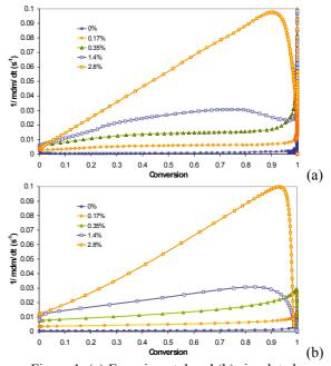
Figure 1. (a) Experimental and (b) simulated instantaneous soot oxidation rate curves as a function of conversion for the case of fuel-borne catalysts
