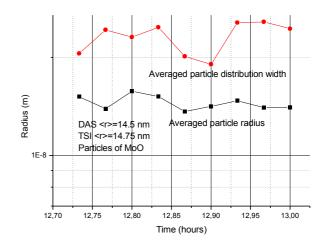
Figure 1. Measurements of particle size distribution made by DAS and DMA.
