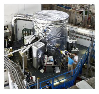
Figure 1: The CLOUD experiment in the CERN PS experimental zone, July 2010. The 3 m stainless-steel CLOUD chamber is enclosed inside the thermal housing visible in the photograph.
