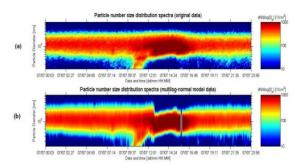
Figure 1: New particle formation event observed on summer period of 2009 at Akrotiri research station, Crete, Greece (a) raw data, (b) data derived from the AMANpsd algorithm.
