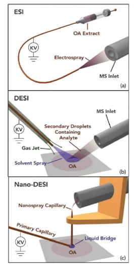
**Figure 1.** Schematics of the sample introduction and ionization setups used for the analysis of OA: (a) direct infusion electrospray ionization (ESI); (b) desorption electrospray ionization (DESI) (c) nanospray DESI. Reproduced from ref. *Nizkorodov et al*, 2011.
