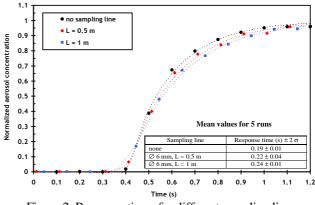
Figure 2. Response times for different sampling lines
