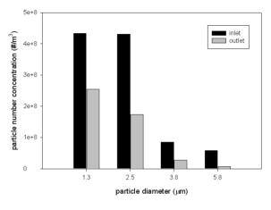
Figure 2. Particle number concentration of axial-flow cyclone inlet and outlet.
