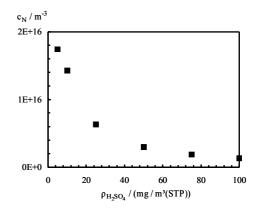
Figure 1. Total number concentration of all droplet classes in the quench column outlet as a function of the  $H_2SO_4$  inlet concentration (Wix 2008)
