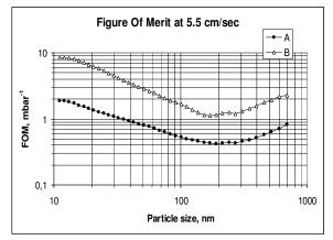
Figure 2. FOM for filters A and B.
