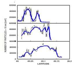
Figure 1. Plume cross sections after 5, 15 and 35 km in a combine power plant / refinery plume (Junkermann et al., 2011).
