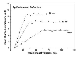
Figure 1. Mean particle charge as a function of impact velocity for silver particles of different size
