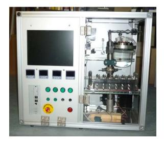
Figure 1. Novel Exposure System for Air Liquid Interface exposure of cell cultures towards particle emissions from biomass burners
