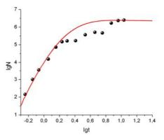
Fig. 1. Time dependence of particle concentration formed in benzaldehyde photolysis. Points – experiment, line – simulation.
