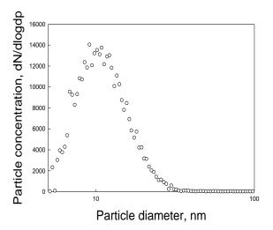
Figure 1. The particle size distribution of ESP generated particle.
