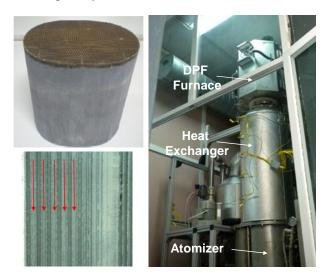
Figure 1. The AID pilot-scale unit. Up-left: a coated oval-shaped DPF. Down-left: the catalyst coating at the inlet channels of the DPF.
