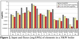
fuelled by spruce wood-chips without and with ESP
