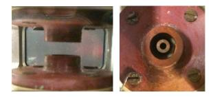
Figure 1. Cylindrical electrodynamic balance. Side view (left) and top-down view (right) of electrodes.
