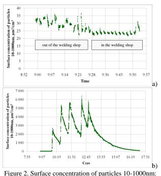
a) background levels out of the welding shop and in the shop, b) before, during and after welding process AERO-TRAK results (A fraction).
