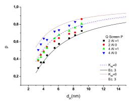
Figure 1. Comparison between experimental penetrations and those calculated with Ec. (3) for 2 and 4 aluminium screens and aerosol flow rates of 2 lmin<sup>-1</sup> and 4 lmin<sup>-1</sup>.
