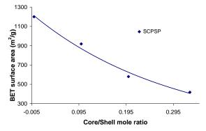
Figure 1. BET surface are with the core/shell ratio for the solid core porous shell particles.
