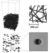
Figure 2 3D model with inflow area (top left), fibres from above (top right), fibres from side (bottom left), electric field computed in the surrounding area of a single bipolar fiber (bottom right).
