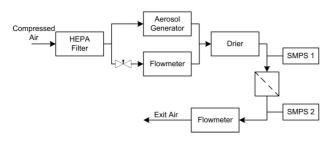
Figure 1. Scheme of the experimental setup.
