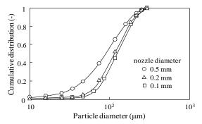
Figure 2. Cumulative size distribution of dry ice particles exhausted from tube (tube diameter = 6 mm, distance from the tube = 40 mm).
