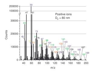
Figure 1. Positive ions measured from 80 nm particles formed from the dark ozonolysis of  $\alpha$ -pinene.
