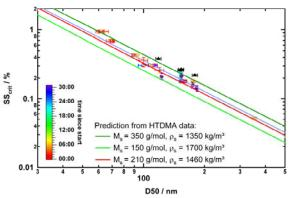
Figure 1. Measured and predicted CCN activation data. The colored dots were measured with the CCN-C (error bars are standard deviation during measurement interval). In black: predicted activation using HTDMA measurements (at 90% RH) and a constant  $\kappa$ . Colored lines: predictions with UNIFAC using different values for molecular mass and density (for details see text above).
