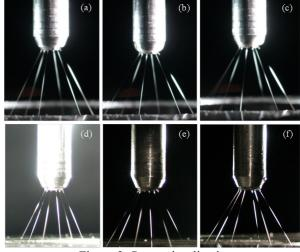
$\begin{array}{l} Figure \ 2. \ Spray \ visualization. \\ (a) \ Q_{ethanol} = 4ml/h, \ Q_{olive \ oli} = 12ml/h; \ (b) \ Q_{ethanol} = 4ml/h, \ Q_{olive \ oli} = 16 \ ml/h; \\ (c) \ Q_{ethanol} = 4ml/h, \ Q_{olive \ oli} = 20ml/h; \ (d) \ Q_{ethanol} = 6ml/h, \ Q_{olive \ oli} = 18ml/h; \\ (e) \ Q_{ethanol} = 6ml/h, \ Q_{olive \ oli} = 24ml/h; \ (f) \ Q_{ethanol} = 6ml/h, \ Q_{olive \ oli} = 30ml/h. \end{array}$
