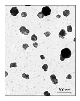
Figure 1. Sample obtained with the AQPS probe at 900°C in biomass post-combustion gases.
