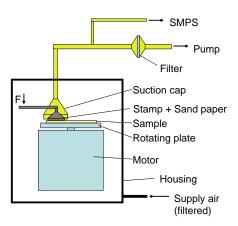
Figure 1: Test rig for abrasion experiments
