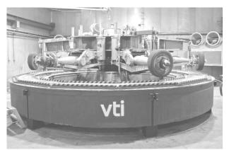
Figure 1. The VTI Road Simulator
