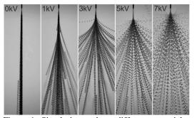
Figure 1: Simple-jet mode at different potentials and constant flow (240 mL/h). The potentials (written on the upper left corners) were applied on the ring while keeping the nozzle (0.41mm OD) grounded. Distance between the nozzle and the ring was kept constant at 2,5cm.
