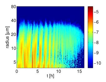
Figure 1. Temporal evolution of the droplet size distribution of iso-C4E1 droplets in water. A slow drift in temperature (25 K in 16 h) causes the system to oscillate.
