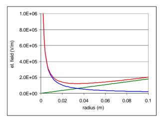
Figure 2. Electrical field due to corona voltage (blue) space charge (green) and total field (red).
