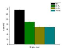
Figure 3. Mean size of the particles emitted as a function of engine load.
