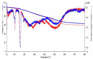
Figure 1. TG curve of NIST 1648 (blue) and NIST 1649a (red) in nitrogen, heating rate 10 °C/min.
