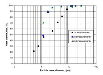
Figure 1. Particle size distribution measured by the Anderson Mark 3 Impactor
