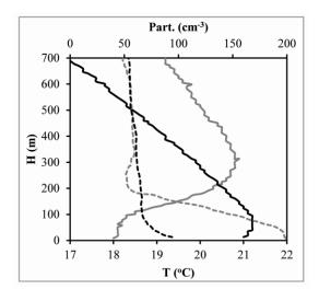
Figure 1. Temperature and particle concentration profiles obtained during the paraglider ascent and descent.
