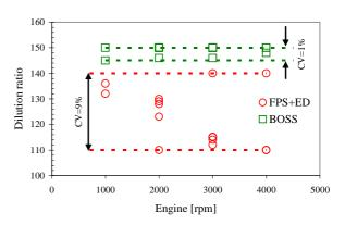
Figure 1. BOSS is compared to a commonly used sampling system, available in the market.
