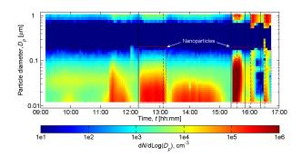
Figure 1: NP emissions from liquid flame spray processes. Red dashed squares shows the fraction of NPs.
