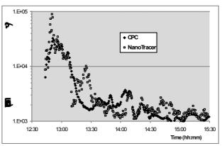
Fig 1: Time series of CPC and Nanotracer measured in a classroom over a two-hour period.
