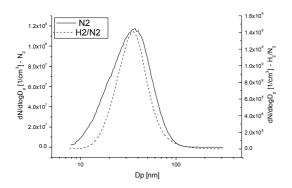
Figure 1. The number size distribution of Cu/Si particles prepared from non-purified precursor and vaporized at the heat bath temperature between 234-239 °C. (Size distribution not dilution corrected, dilution ratio 1:19).
