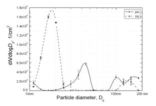
Figure 2. Dependence of generated particle size distribution on laser pulse energy during the ns and ps laser ablation of nickel **in the argon gas**.
