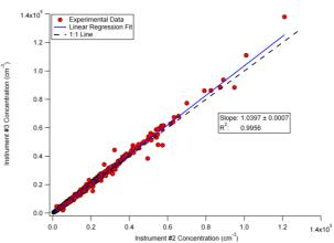
Instruments were tested with a number of different wick materials and with water of different qualities (e.g. distilled water, tap water, etc.). The instruments were challenged with both indoor and outdoor air, and were subjected to a number of real-world conditions, such as water deprivation to test the ability to recover from these incidents.
