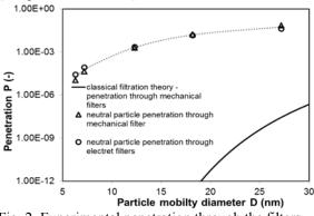
Fig. 2. Experimental penetration through the filters
