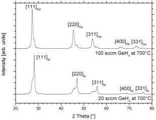
Figure 1. XRD data for Si-Ge composite material.
