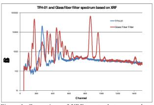
Figure 1. Comparison of XRF spectra between a glass fiber filter and TFH-01.
