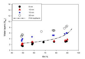
Figure 2 Number of the water layers versus RH at selected dry particle diameters for atomized fumed SiO2 and the fitted FHH-isotherm.
