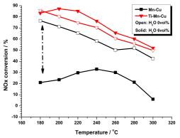
Figure 1. NOx conversion over Mn-Cu and Ti-Mn-Cu catalysts. Reactants: 800ppm NO, 800ppm NH<sub>3</sub>, 3 vol.% O<sub>2</sub> and 0, 6 vol.% H<sub>2</sub>O. GHSV was 60,000 hr<sup>-1</sup>.
