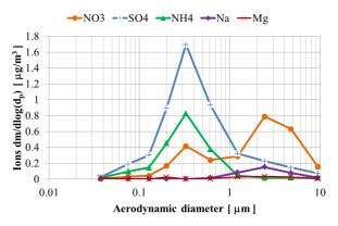
Figure 1. The mass size distribution of main ions from BLPI measured next to the freeway (Sep 2008).
