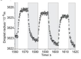
Figure 1. Change in droplet radius with time. Grey shaded regions show when the heating beam is on.
