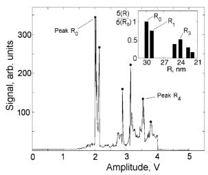
Figure. 1. Resulting rupture signal versus voltage supplied to the quartz resonator. The resulting particle size distribution is shown in the insert.
