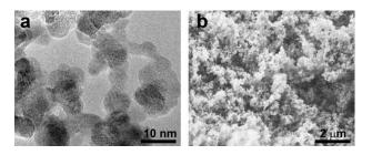
Figure 1. (a) TEM and (b) SEM images of NaYF<sub>4</sub>:Yb,Tm nanoparticles.
