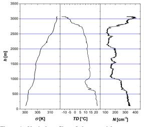
Figure 1: Vertical profiles of the potential temperature  $\Theta$ , the dewpoint temperature *TD*, and total particle number concentration *N* during ascent on November 21, 2010.
