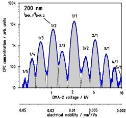
Figure 1. mobility spectrum of a pre-classified (200nm) and neutralized sodium chloride aerosol measured by a CPC after DMA-2 in a TDMA setup. i indicates the state of charge in DMA-1 and DMA-2, respectively.
