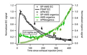
Figure 1. Soot and organic signal during an experiment were diesel exhaust spiked with toluene and m-Xylene was irradiated with UV.
