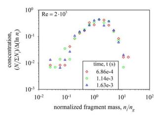
Figure 1. Steady state agglomerate mass distribution at three different simulation times. An equilibrium between coagulation and break-up is reached.
