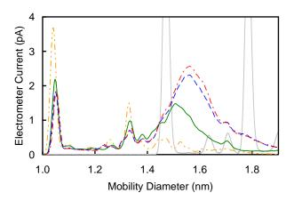
Fig. 1. Size spectra of oxytocin before addition of TCEP (solid green) and 30 min (long dash blue) and 2 hours (alternating dash red) after TCEP addition, each in ammonium acetate solutions (short dash orange). THAB (grey dotted) was used to calibrate the distributions.
