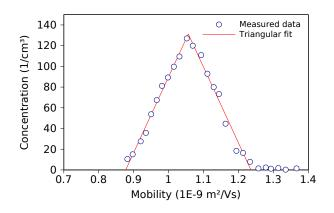
Figure 1: Experimentally found DMA TF and triangular fit ( $R^2 = 0.990$ ).
