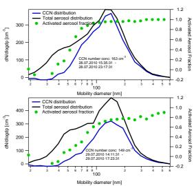
Figure 1: Two examples total and CCN number size distributions, along with the activated number fraction.
