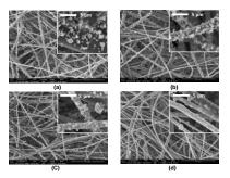
Figure 1. SEM images of (a) RH 25% (b) RH 57% (c) RH 82% (d) RH 90%
