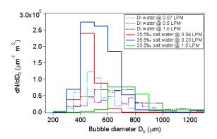
Figure 1 Preliminary photograph-analyzed bubble size distributions for the frit placed in the bottom of the tank.
