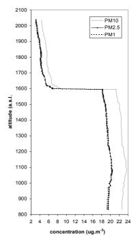
Figure1: Vertical profile of PM concentrations above Svratouch station.
