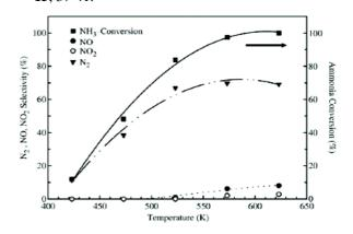
Figure 1. Relationship of the ammonia conversion, N<sub>2</sub>, NO and NO<sub>2</sub> yield at various temperatures over the Pt-Pd-Rh nanoparticles cordierite substrate catalyst. Test conditions: 800 ppm NH<sub>3</sub> in He, O<sub>2</sub> = 4%, RH=12%, Temperature = 423-623 K, GHSV = 92000 hr<sup>-1</sup>.
