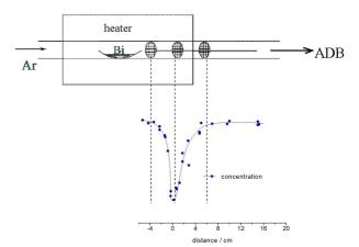
Fig. 3. Experimental determination of nucleation position inside the flow reactor.
