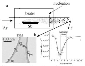
Figure 1. a) Experimental setup b) TEM image of aggregates c) Illustration of the "supersaturation cut-off" method.
