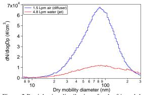
Figure 2 Particle size distributions for the frit and the plunging jet for artificial sea water of salinity 35‰.
