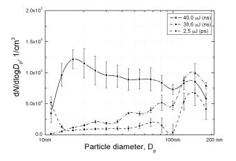
Figure 1. Dependence of generated particle size distribution on the laser pulse energy during the ns and ps laser ablation of nickel **in the ambient clean air**.
