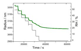
Figure 2. Time dependence of the size of a sucrose droplet (green) with change in RH (grey line, right axis). Adapted from (Tong, *et al.* 2011)
