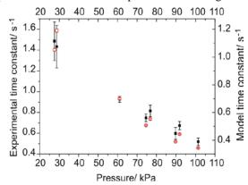
Figure 2. Experimentally measured pressure dependence of the condensational growth time constant (squares) compared with model predictions (circles) for  $\alpha_m = \alpha_t = 1$  using the model of Kulmala *et al.* (1993). Proportional change on each axis is the same.
