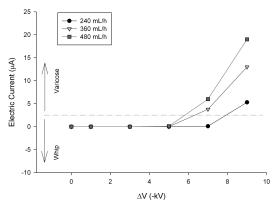
Figure 2: Applied potential against spray electric current for three different flows (240, 360 and 480 mL/h). The arrows and dotted line were arbitrary placed to show the varicose break-up and the whipping break-up regions.
