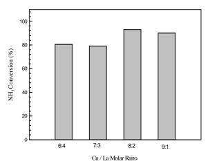
Figure 1. Effect of the metal content on the Cu-La nanomaterials in the conversion of NH<sub>3</sub>. Test conditions: 1000 ppm NH<sub>3</sub> in He,  $O_2 = 4\%$ , temperature = 400°C, RH = 12%, GHSV = 92000 ml/h-g.
