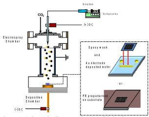
Figure 1. Schematic diagram of sensor fabrication setup
