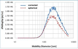
Figure 1. Spherical and corrected aggregate number size distribution, example taken from condition C.4
