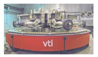
Figure 1. Experimental setup for emissions of the interaction between tyre and pavement.
