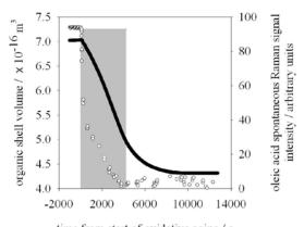
time from start of oxidative aging / s Figure 1: Decrease in OL signal (open circles, right axis) and decrease in size (black squares, left axis) revealing the reaction kinetics and particle-vapor partitioning
