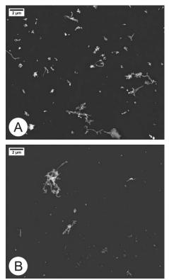
Figure 1. Examples of sampled CNF (A) and CNT (B) fibres.
