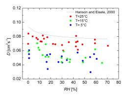
Figure 1. Diffusion coefficient data of  $H_2SO_4$  in air as a function of relative humidity (RH) at three temperatures 5, 15 and 25 °C compared to fit to  $H_2SO_4$ -N<sub>2</sub> data of Hanson and Eisele, 2000.
