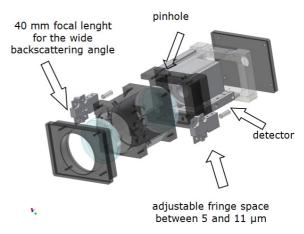
Figure 2. Design of the LDA probe head
