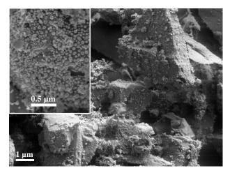
Figure 2. SEM micrograph of copper coated silicon particles. The insert shows the coating particles in more detail.
