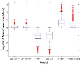
Figure 1. Box-whisker plot showing how changing the vapour pressure input data affects the SOA condensed mass. Base case is vapour pressure by N/N-VP, ideal liquid behaviour and no hydrolysis of anhydrides. SB and JR refer to boiling point estimation by Stein and Brown and Joback and Reid respectively, MY refers to the vapour pressure correlation of Myrdal and Yalkowsky. The sixth plot refers to the effect of hydrolysing all acid anhydrides, while retaining base case values for the other inputs.
