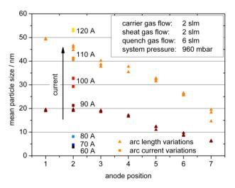
Figure 2. Influence of arc length and arc current on mean particle sizes (SMPS-measurement).
