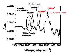
Figure 1. A Reflection-Absorption Infrared spectra (RAIR spectra) of  $C_{60}$  aerosol exposed to ozone.
