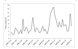
Figure 1. The water content of aerosol samples at RH=50% relative to RH=20%
