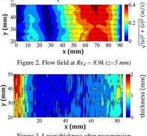
Figure 3. Layer thickness after resuspension at  $Re_d = 27.2k$
