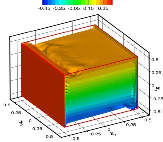
Figure 1. Time-averaged dimensionless temperature profile of DHC, acquired with DNS (Puragliesi, 2010).
