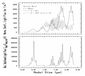
Figure 1. Normalized scattering light flux for scattering angles  $\theta = 20^{\circ}$  and  $170^{\circ}$  (upper graph) and their ratio (lower graph) both as a function of modal size.
