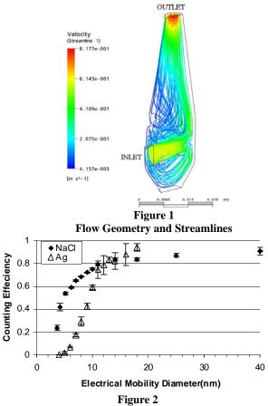
**Counting Efficiency for NaCl and Ag Particles**
