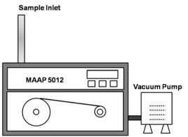
Figure 1. The schematic of Multi Angle Absorption Photometer (MAAP)
