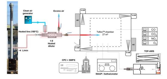
Figure 1. Schematic representation of the inlet system and smog chamber setup (Heringa et al 2011).
