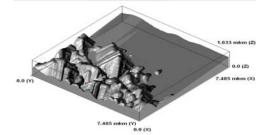
Fugure2. The example of the distribution of nanoparticles on the filter.
