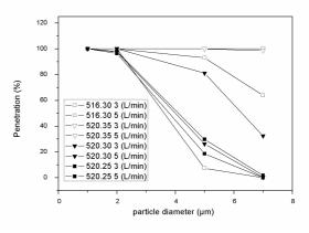
Figure 1.The penetration of the aerosol particles in the function of particle diameter.
