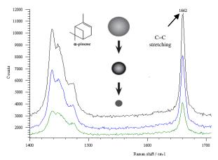
**Figure 2.** An example of evaporation of a levitated  $\alpha$ -pinene droplet in nitrogen at a relative humidity, RH, of 50% and T = 25 °C recorded by Raman spectroscopy as a function of time (acquisition time of 60 s).
