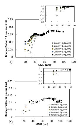
Figure 1. Calculated bounce factors for the 17 nm size limit measured for a)  $O_3$  initiated oxidation and b) OH dominated oxidation in presence of SO<sub>2</sub>. Density values  $0.8 - 2 \text{ g/cm}^3$  were used in calculations. Insets in the upper right corners of figures a and b show details in bounce factor values for the smallest particles.
