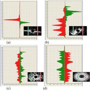
Figure 2. Examples of APC CMOS-array data for various particle morphologies: (a) columnar, (b) platelike, (c) irregular cubic, (d) droplet. Y-axis represents array 0-512 pixels; x-axis represents light intensity for each array. (Image inserts are from SID3 probe data for similar particle types).
