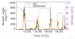
Figure 3. Time series of aerosol mass derived from CAS (black) and nephelometer scattering measurements (orange). The aircraft altitude is shown in purple.
