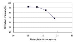
Figure 3. Effect of plate-plate distance on collection efficiency.
