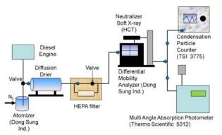
Figure 1. The schematic of experimental apparatus used in the present study.
