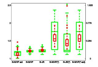
Figure 1. Predicted growth factors and kappa kohler values as a function of predictive technique and number of compounds used in the partitioning calculations. 10000 compound simulations are shown as red boxes, 2 compound simulations as green. Predictive technique acronyms displayed on the x axis, (\*) denotes assumed evaporation of all semi-volatiles on drying. The left-hand y-axis lists calculated GF, the right side lists the corresponding kappa kohler values.
