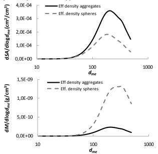
**Figure 2**. Distributions of surface area (*SA*) and mass (*m*) assuming either spherical or aggregated particles.
