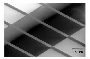
Figure 1. Scanning electron microscopy image of silicon nitride string resonators.
