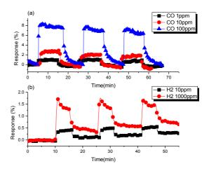
Figure 2. Gas sensor response for CO and H<sub>2</sub> gas
