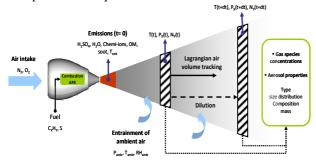
Figure 1. Scheme of the modelised aircraft plume.
