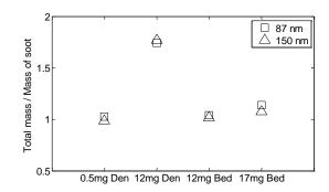
Figure 2. Ratio between obtained total mass and mass of soot core using different inlet DOS concentration for denuder (Den) and packed bed (Bed)
