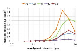
Figure 2. The mass size distribution of main elements from BLPI measured next to the freeway (Sep 2008).
