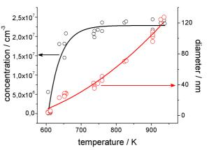
Figure 2. Aerosol concentration and aggregate size vs heating temperature.
