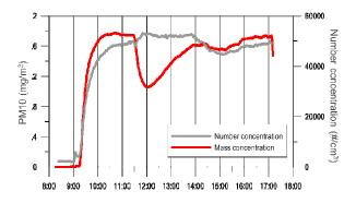
Figure 4. Concentration of particulate mass (PM10) and number concentration when CMA is applied in the road emission experimental setup.
