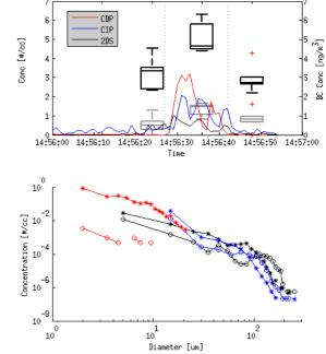
Figure 1. a) Concentration of particles detected by the 2DS (black), CIP (blue) and CDP (red). Also box and whiskers for the total scattering particle concentration (black) and total black carbon number (grey) from the SP2. b) Averaged size distribution for the regions indicated by the box plots in part a: within the contrail (stars), at the contrail edges (circles).
