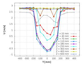
Figure 2. Horizontal LDA profiles of wind speed (U) at different heights, X = 80 mm from the model.
