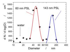
Figure 3. Size distribution of 60 nm and 143 nm PSL particles mixture, measured by WRAS. Dots - experimental results, lines – log-normal fits.
