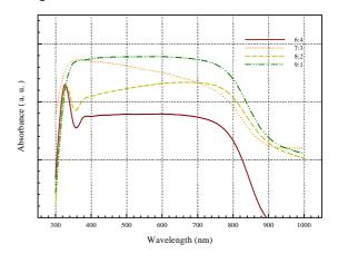
Figure 2. A UV-Vis absorption spectra of various metal content on the Cu-La nanomaterials for the conversion of NH<sub>3</sub>. Test conditions: 1000 ppm NH<sub>3</sub> in He,  $O_2 = 4\%$ , RH = 12%, GHSV = 92000 ml/h-g.
