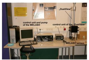
Figure 1. Modified version of the Palas DustView®, including single-drop apparatus and OPC "WELAS®"
