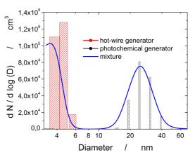
Figure 2. Size distributions of two individual aerosols and their mixture, measured with NADB. Red bars – aerosol from hot-wire generator, (Ankilov *et al.*, 2002), black bars – aerosol from photochemical aerosol generator (Dubtsov, 1996), line– mixture.
