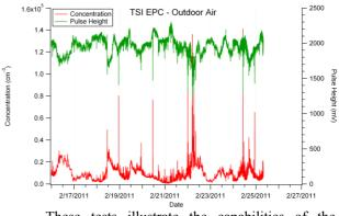
These tests illustrate the capabilities of the Model 3783 EPC for long-term monitoring. The instruments have been shown to run autonomously for at least a month, providing accurate particle concentration measurements with high time resolution.
