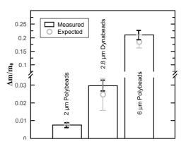
Figure 3. The average measured mass ratios for the three different types of micro particles compared to the expected values.
