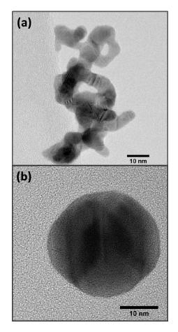
Figure 1. Gold nanoparticles of the same mass (0.24 fg)(a) before and (b) after reshaping. The mobility diameter decreased from 60 to 31 nm upon reshaping.
