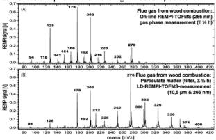
Figure 1: REMPI mass spectra from wood combustion gas-phase (online REMPI-MS measurement) and from the filter used for hot-gas particle precipitation (off-line, laser desorption-REMPI-MS) [1].
