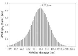
Figure 1. The mobility size distribution of airborne MWCNTs in IPA solvent.
