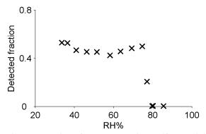
Figure 2 Fraction of 91nm ammonium sulfate particles detected after impaction with varying humidity
