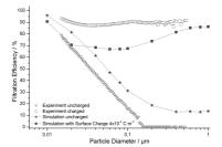
Figure 3 Comparison of measured and simulated fraction filtration efficiencies.
