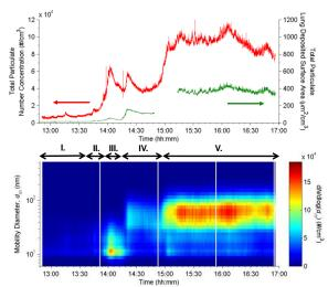
Figure 1. Measurement for air-borne particles during the extrusion operation for CNT-imbedded nanocomposites. Upper panel shows the total number concentration and lung-deposited surface area concentration; lower panel shows the evolution of the particle number-size distribution.
