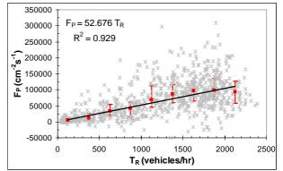
Figure 1. Aerosol fluxes against traffic rate. Red squares are median values calculated in bins of 250 vehicles/hr and error bars represent the IQR.
