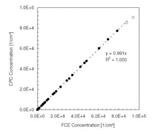
Figure 1. Linearity of the PMP-CPC. Open symbols are not included in the linear regression.
