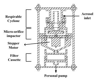
Figure 1 Schematic diagram of the IOSH-NCTU PNS.
