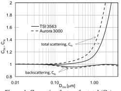
Figure 1. Correction factors for total  $(C_{ts})$  and backscattering  $(C_{bs})$  versus the volume median diameter.
