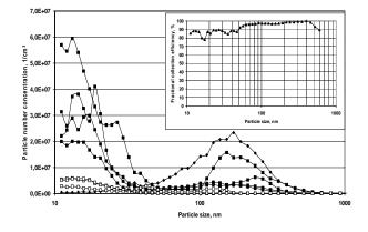
Figure 1. Size distribution of wood combustion aerosol (closed – raw gas, open – clean gas) and fractional collection efficiency of the high temperature electrostatic precipitator
