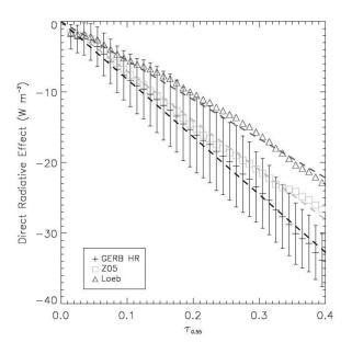
Figure 1. SW Direct Radiative Effect as a function of aerosol optical depth at 0.55 microns ( $\tau_{055}$ ). GERB HR indicates the original GERB fluxes, Z05 and Loeb are fluxes obtained using the Zhang *et al* ADMs and Loeb *et al* aerosol correction method respectively
