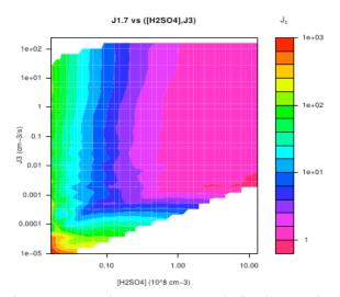
Figure 1. Example AeroCLOUD-calculated corrections for  $J_{2.5}$  values (ie. detection with a 2.5nm-threshold CPC). The colour contours relate sulphuric acid concentration (x axis) and  $J_{2.5}$  (y axis) with a correction factor that ranges from 1 (plotted in blue-magenta) for high [H<sub>2</sub>SO<sub>4</sub>] up to 1000 (plotted in orange-red) for low [H<sub>2</sub>SO<sub>4</sub>] and low  $J_{2.5}$  values.
