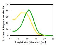
Fig. 2, cloud droplet size distributions in nonprecipitating stratocumulus clouds under low (green) and slightly enhanced CCN number concentrations (Junkermann et al., 2009)
