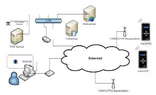
Figure 1: Structure of the miniDiSC measurement network.
