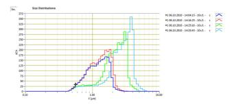
Figure 1. Working fluid butanol. Particle size distributions of droplets resulting from changed saturator and condensor temperatures.
