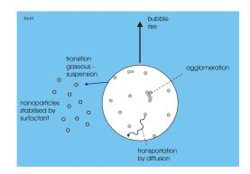
Figure 1: Transfer steps of gas-borne nanoparticles.
