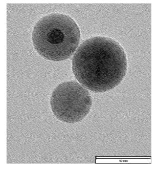
Figure 2. Freshly- to medium-aged Al aerosol. The Al nanoparticles appear as spheres from 20 to 40 nm.
