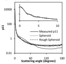
Figure 2. Measured phase function for the particle shown in Figure 1, along with RTDF calculations for a smooth spheroid and a rough spheroid. The refractive index used in the calculations was 1.55 + 0.003i.
