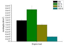
Figure 2. Mean number concentration of particles emitted as a function of engine load.
