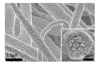
Figure 3: Aerosol derived calcium phosphates are smoothly incorporated in polymer fibres and showing a highly reactive phase.
