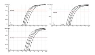
Figure 2. PCR amplification of phages MS2 (A), T4 (B) and their mixture (C) collected from the aerosol stream. PCR assays were performed in duplex format.
