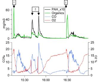
Figure 1. Time resolved total organics, PAHs, CO and  $O_2$  during high load in the wood stove. "1" denotes addition of full batch on glowing embers. "2" denotes addition of 1/3 batch in flaming phase.
