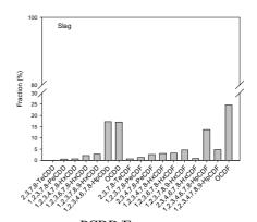
PCDD/F congeners Figure 1. Congener profiles of PCDD/Fs in the slag after thermal treatment of EAF ash at 1450 °C.
