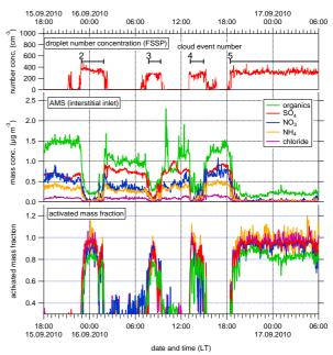
Figure 1. Example for the activated mass fraction analysis during selected cloud events. Upper panel: cloud droplet number concentration, middle panel: absolute mass concentrations (interstitial inlet), lower panel: activated mass fractions.
