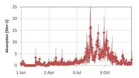
Figure 2. Daily averages of absorption coefficients measured at 637 nm from Feb 2008 to Dec 2010.
