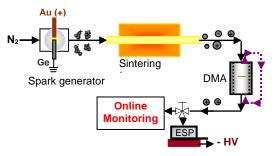
Figure 1. Schematic representation of different components utilized to prepare AuGe nanocomposites.
