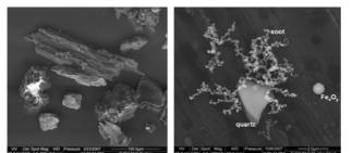
Figure 1. a) Backscatter electron image of a lignite particle; b) Secondary electron image of a soot, quartz and iron oxide particle.
