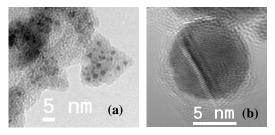
Figure 2. HRTEM images of synthesized AuGe nanocomposites prepared at spark frequencies of (a) 55 and (b) 74 Hz.
