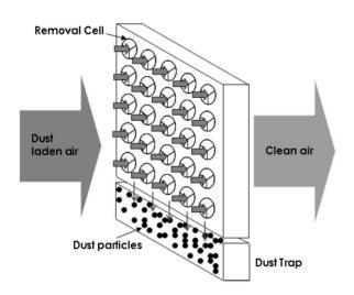
Figure 1. Schematic of air filter system of axial-flow cyclone.
