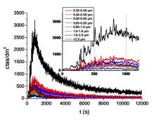
2. Time evolution of Aerosol particle size measured with OPC
