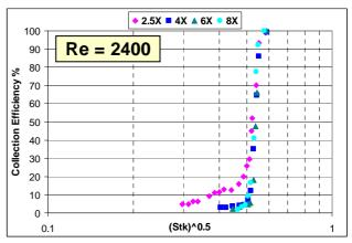
Figure 2: Collection efficiency curves Re = 2400
