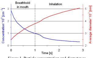
Figure 1. Particle concentration and diameter as functions of inspiratory time.
