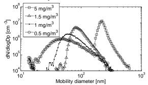
Figure 1. Effect on particle size distribution by allowing different amounts of DOS and constant amount of KCl  $(0.5 \text{ mg/m}^3)$  enter the denuder at 1 lpm.
