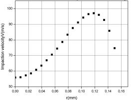
Figure 2. The impaction velocities of 60nm particles as a function of the radial distance from the axis of the jet.
