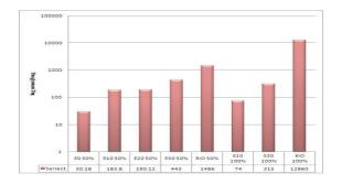
Figure 1: Average ROS concentrations for different fuel and load settings. Note that concentrations of ROS per mg of particulate matter are presented on a logarithmic scale.
