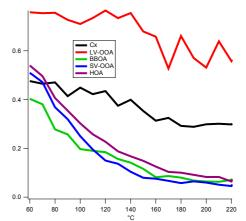
Figure 2: Thermodenuder relative attenuation for carbon clusers (Cx), Low Volatility Oxidised Organic Aerosol (LV-OOA), Biomass Burning OA (BBOA), Semivolatile OOA (SV-OOA) and Hydrocarbon-Like OA (HOA).
