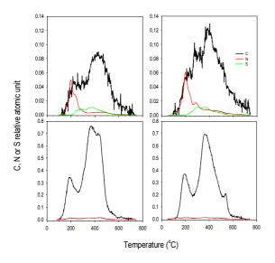
Fig. 1. The MESTA thermograms of the ambient PM (top) and those of biomass burning emitted (bottom).
