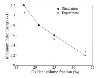
Figure 1. MPE of laser-induced detonation depending on oxidant volume fraction.
