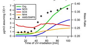
Figure 1. Chemical composition during an exhaust ageing experiment. The increase in AMS/SMPS mass ratio is likely due to an increase in  $E_b$  of the sampled aerosol. The time trace of SO<sub>4</sub> supports this.
