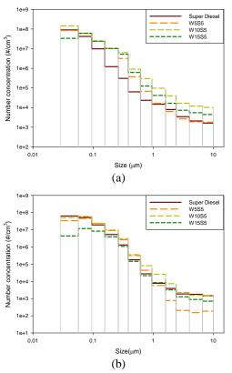
Figure 2.Particle size distribution of exhaust from a diesel engine generator as different fuel at (a)0W; (b)3600W.
