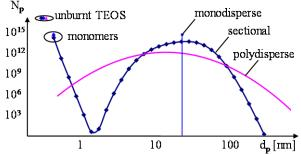
Figure 2. Particle size distribution at the symmetry axis of the facility (Fig. 1) performed with the monodisperse, the poldydisperse and the sectional model (Giglmaier, 2010)
