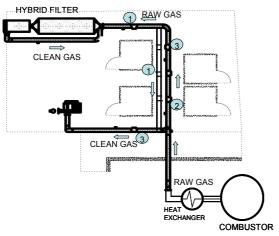
Figure 1. Validation test line lay-out. Sampling ports for aerosols (1), dioxins (2) and gases (3)
