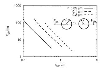
Figure 1. Relative photophoretic interaction force between two identical spherical particles of various sizes versus distance.
