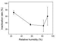
Figure 2. Variation of inactivation rate of antimicrobial filters using natural product nanoparticle under RH surrounding conditions.
