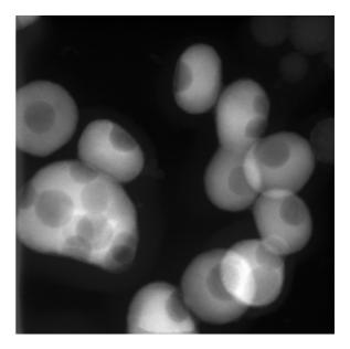
Figure 2. STEM picture of Si-Ge core-shell structures (dark: Si, bright: Ge).
