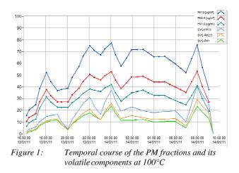
The temporal resolution is 6 seconds. By limiting the size channels, measurements can be executed at 1 Hz, which enables the application of the Eddy-Correlation calculation for determination of aerosol flows.
