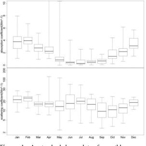
Figure 1. A standard box plot of monthly aerosol absorption coefficient (top) and scattering coefficient (bottom) at 574 nm as derived from daily average for 50m height level taken over the time period October 2006 through April 2010.
