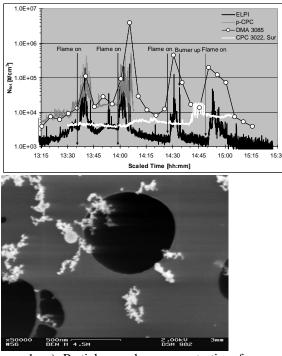
Figure 1: a) Particle number concentration for n-HALO<sup>®</sup> inside the process enclosure and in the surroundings (white curve, scaled time) b) A scanning electron microscope (SEM) micrograph of the collected nanoscale particles from inside the enclosure. Particles were mainly aggregates, primary particle size approximately 20-30 nm.
