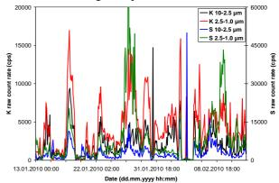
Figure 2. Selection of two-hourly size-segregated elemental amounts for potassium (K) and sulphur (S), measured by RDI-SR-XRF at IPSL/SIRTA in Paris (France).
