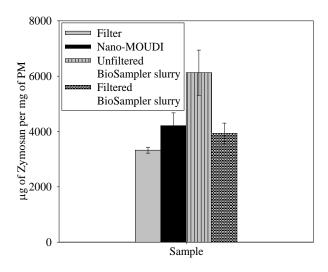
Figure 1. ROS response of the water extracts of the filter and Nano-MOUDI  $PM_{2.5}$  samples as well as the unfiltered and filtered BioSampler  $PM_{2.5}$  slurry. Error bars represent one standard error.
