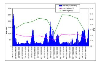
Figure 1. PM<sub>10</sub>, PM<sub>2.5</sub> and natural radiation (28 Oct. 2008 - 8 Nov. 2008).
