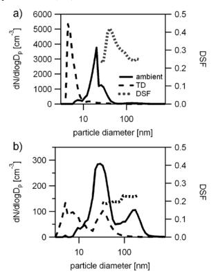
Figure 1. The descriptive shrinking factor DSF, and aerosol number size distributions at ambient temperature and after TD treatment: a) OW and b) PIZ.
