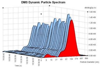
Figure 1. Count size distribution of the aerosol obtained in the case of combustion of PA-6 filled with CNT
