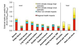
Fig 3. External costs per MJ useful heat for wood and fossil fuel systems in Switzerland.[3]
