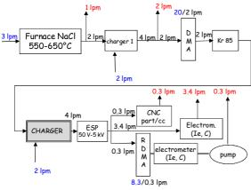
Figure 1. Setup for monodisperse aerosol generation and charge distribution measurements
