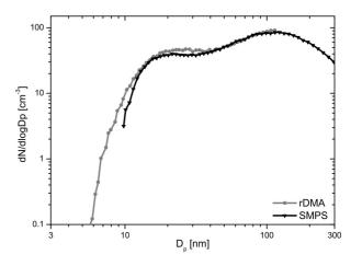
Figure 1. Preliminary intercomparison between our rDMA and a scanning mobility particle sizer (SMPS) at ambient air.
