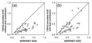
Figure 1. Correlations between CMAQ-simulated AOD and AERONET AOD in spring, 2006: (a) CMAQsimulated AOD without dust contributions vs. AERONET AOD and (b) CMAQ-simulated AOD with dust contributions vs. AERONET AOD.
