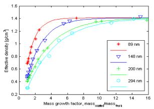
Figure 1. The measured and fitted curve for the effective density as a function of the mass growth factor (*Gfm*). The following fit was used  $\rho_{eff}(d_{me}) = \rho_{fresh}(d_{me}) + (1.4 - \rho_{fresh}(d_{me}))(1 - exp((Gfm - 1)/a(d_me)))$
