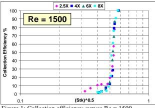
Figure 1: Collection efficiency curves Re = 1500
