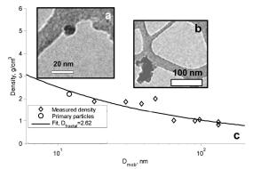
Figure 1 (a) TEM images of smaller spherical and (b) larger agglomerated fumed SiO2 nanoparticles. (c) Measured effective density versus particle size of atomized SiO2 nanoparticles and fitted density profile with Df= 2.62 (solid line).
