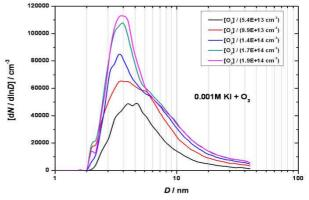
Figure 3. Iodine oxide particle (IOP) formation due to the uptake of  $O_3$  by an I<sup>-</sup> solution.
