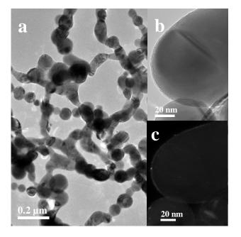
Figure 1. TEM micrograph of copper coated cobalt particles (a). Insert b) shows a coated Co particle at higher magnification. In c) the corresponding dark field image indicates the copper coating on the particle surface.
