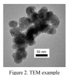
Figure 1 shows an example for UNPA size distribution correction due to particle structure. UNPA measurements also indicate that the analyzed Siparticles have a relatively open structure, as confirmed by TEM images (see Figure 2). Mean *primary* particle sizes reported by UNPA were around 25 nm (C.2 to C.5) and
