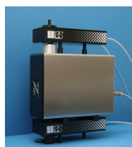
Figure 1. CNC-06 with two welas® sensors for measurement within the system welas® 3000
