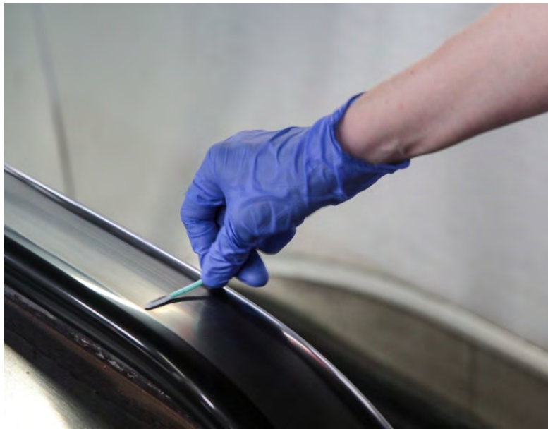
Abbildung 5.1: Sampling the handrail of an escalator in the subway system
