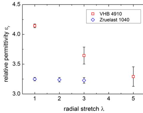
**Figure 5: Relative dielectric permittivity @ 1 kHz of VHB and rubber versus stretch ratio. While VHB shows a stretch dependent permittivity, the permittivity of rubber is insensitive to stretch.**
