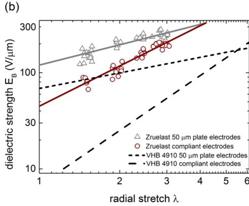
**Figure 4: Experimental values for the dielectric strength  $E_{EB}$  of VHB 4910 (a) and ZRUELAST natural rubber (b) using compliant and rigid electrode configurations. The data are fitted to  $E_{EB}(\lambda) = E_{EB}(1) * \lambda^R$ .**
