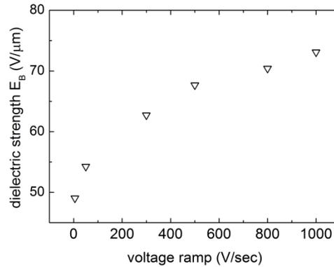
**Figure 3: Breakdown field strength versus voltage ramp, showing an increase of the breakdown field strength with increasing voltage sweep rate.**
